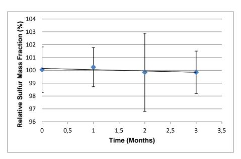
Figure 10. Graph for long term stability of UME CRM 1203-1 at 4 °C
