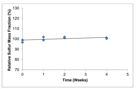
Figure 8. Graph for short term stability of UME CRM 1203-2 at 35 °C
