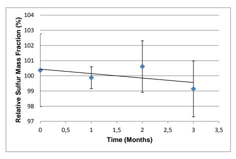
Figure 11. Graph for long term stability of UME CRM 1203-2 at 4 °C
