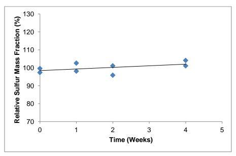
Figure 9. Graph for short term stability of UME CRM 1203-2 at 50 °C
