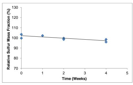
Figure 4. Graph for short term stability of UME CRM 1203-1 at 18 °C
