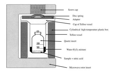
Figure 1. Microwave vessels as used for the decomposition of diesel samples
