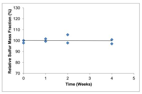
Figure 7. Graph for short term stability of UME CRM 1203-2 at 18 °C
