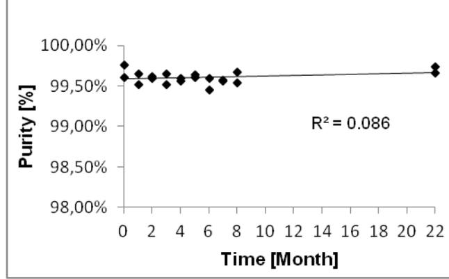
**Figure 4.** Regression analysis with long term stability data.
