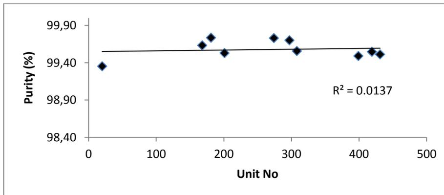
**Figure 2.** Measurement results for homogeneity assessment.
