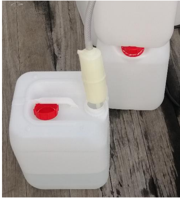
Figure 3. Direct filtration of sampled seawater using Pall AcroPak 1500 0.8/0.2 \mu\text{m} filters
